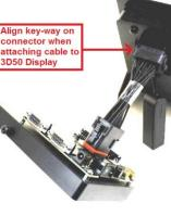
Match Pin 1 on cable to Pin 1 on board
