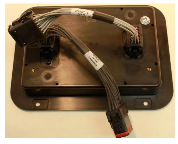
5. Attach the mounting frame with the 3D50 Display to the development stand and secure by installing the lower two screws and washers through the tabs on the development stand, through the back of the mounting frame, and into the back of the 3D70 Display.
