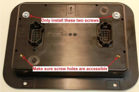
4. Connect the two 18pin DT cables to the back of the display. Note that the cables are different! Match up the keying tabs to insure that the correct cable is installed in the correct connector on the back of the 3D70 Display. The cable marked 3DHH1976-A (typically made with black wires) connects to connector "A" and the cable marked 3DHH1976-B (typically made with gray wires) connects to connector "B".
