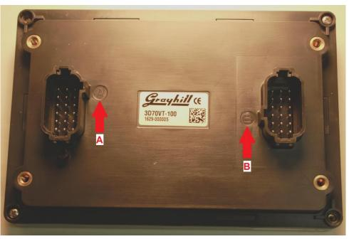
Notice that the 3D70 Mounting Frame has two openings on the back and that one is larger than the other. Place this mounting frame on top of the 3D70 Display with the larger opening to the left (over the connector marked "A").
