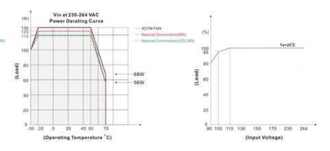
If input voltage is lower than 115VAC, please refer to the output derating V.S. input voltage curve for details
