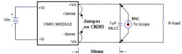
Output ripple and noise measured with 1uF ceramic capacitors across output. A 20 MHz bandwidth oscilloscope is normally used for the measurement.
