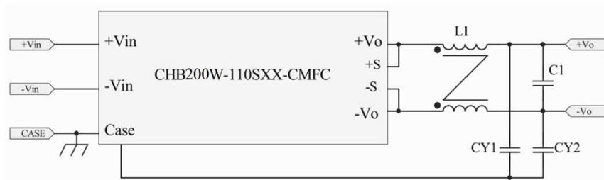
Connection circuit for EMI testing
