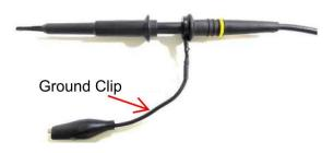
Another method is shown in below, in case of coaxial-cable/BNC is not available. The noise pickup is eliminated by pressing scope probe ground ring directly against the -Vout terminal while the tip contacts the +Vout terminal. This makes the shortest possible connection across the output terminals.
