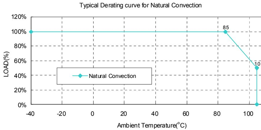
Figure4 Typical Power De-rating Curve for EC2SANH Series
