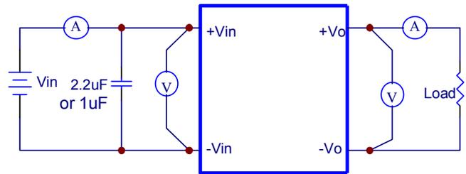
Figure6 EC2SANH Series Single output Test Setup
