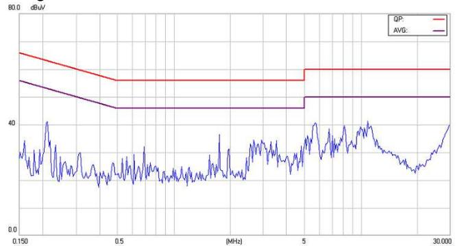
Figure14-2 EMI Conducted Class B for EC2SA03NH
