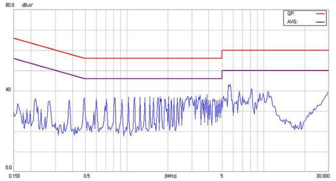
Figure16-2 EMI Conducted Class B for EC2SA05NH
