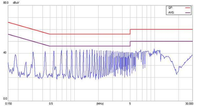
Figure24-2 EMI Conducted Class B for EC2SA21NH
