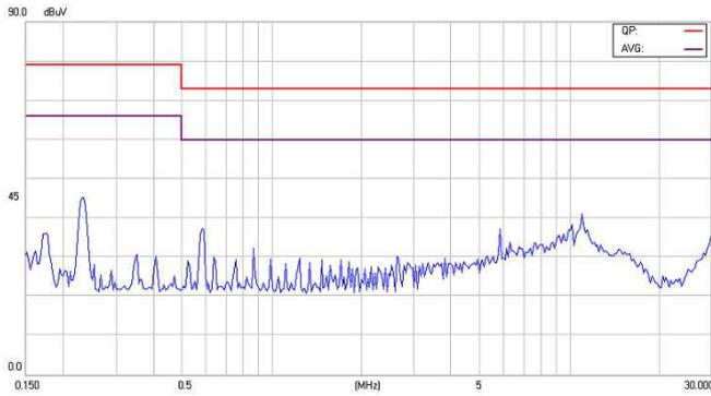
Figure28-1 EMI Conducted Class A for EC2SA25NH
