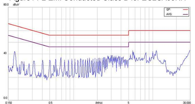
Figure15-2 EMI Conducted Class B for EC2SA04NH
