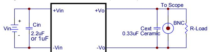
Figure8 Output Voltage Ripple and Noise Measurement Set-up for Single Output
