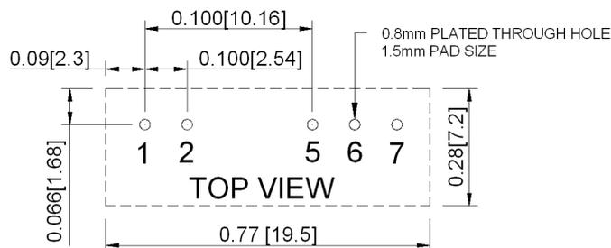
Note: Dimensions are in inches(millimeters)
