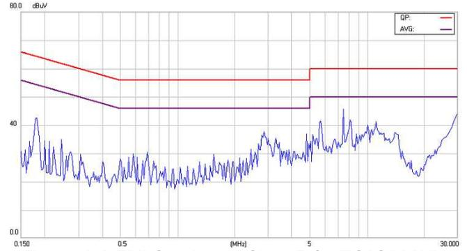
Figure13-2 EMI Conducted Class B for EC2SA02NH
