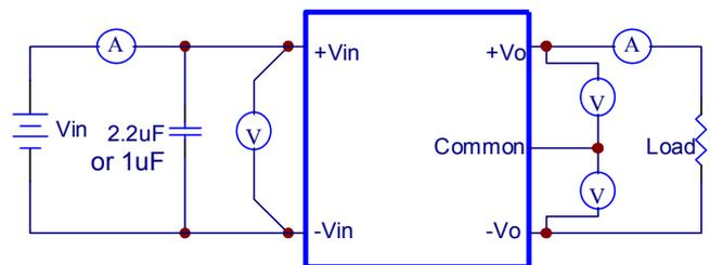
Figure7 EC2SANH Series Dual output Test Setup
