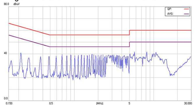
Figure18-2 EMI Conducted Class B for EC2SA11NH
