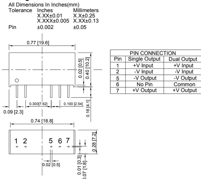
Figure30 EC2SANH Mechanical Outline Diagram
