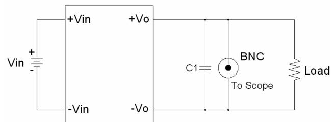
Figure9 Using BNC to Measure Output Ripple and Noise
