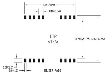
Figure5 Recommended PCB Layout Footprints for SMD packages
