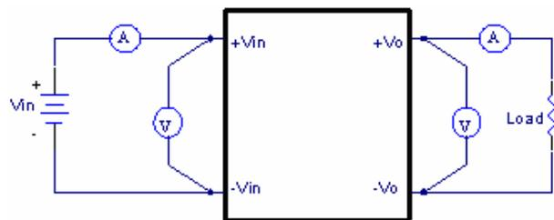
Figure8 EC4AW Series Test Setup
