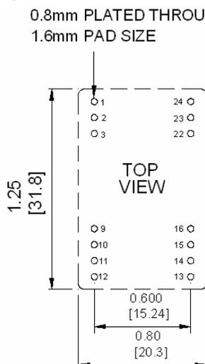
Note: Dimensions are in inches (millimeters)
