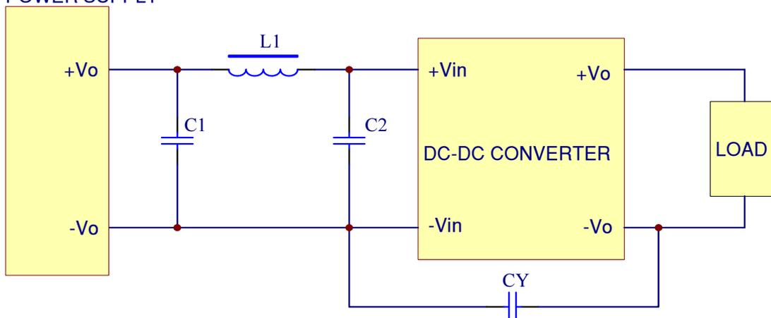
Figure12 Connection circuit for conducted EMI testing
