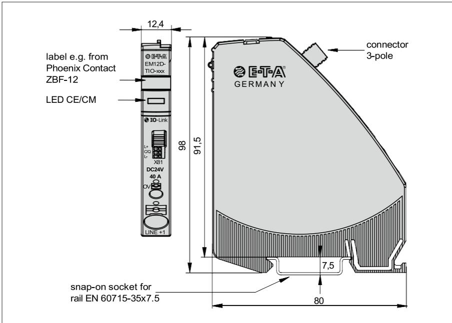
Figure 2: Dimensions of the EM12D-TIO
