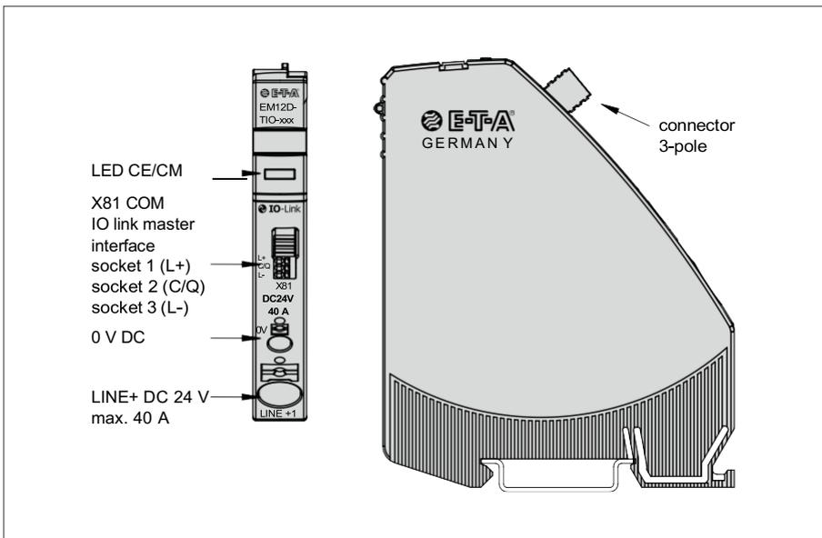
Figure 3: EM12D-TIO status indication and terminals
