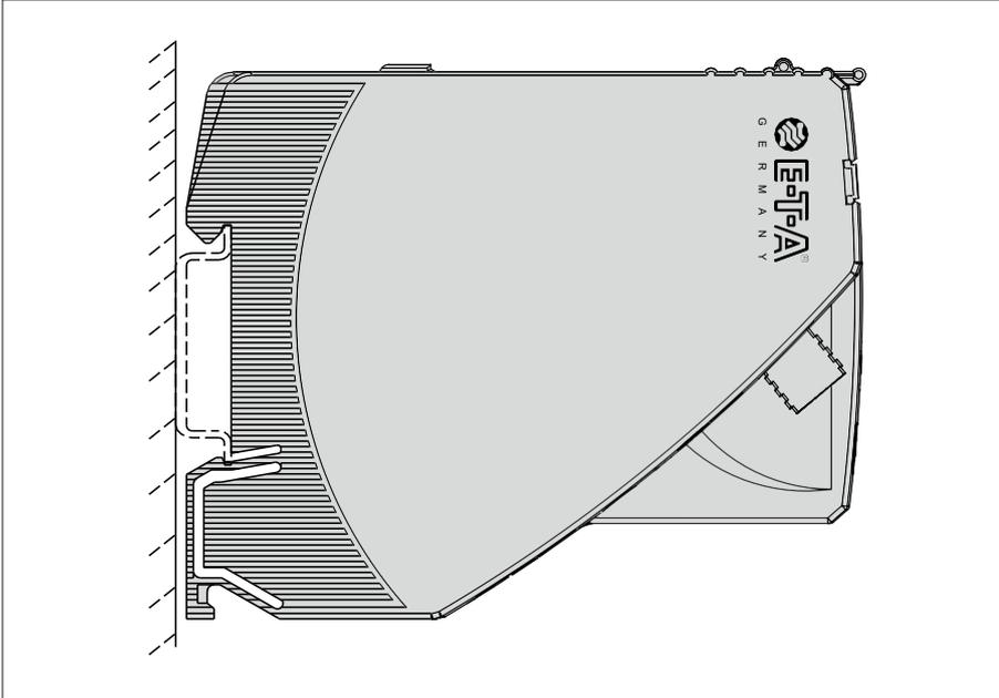
Figure 6: Mounting position of the EM12D-TIO
