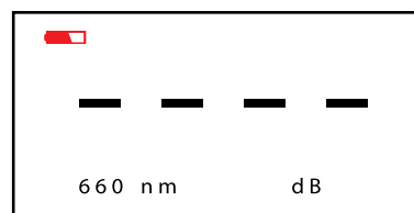
Pic. 6 Power meter display, low battery power
